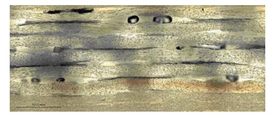
Fig.1. Macrograph of composite structural element, comprising delamination defects (From the site <u>http://www.medus.com.ua</u>)
