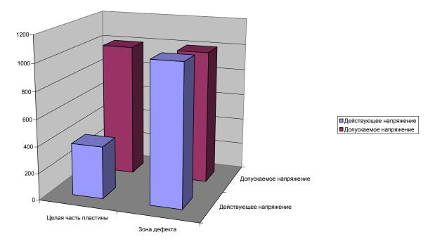
Comparison of stresses on the whole area of the new composite plate and in the defect area
