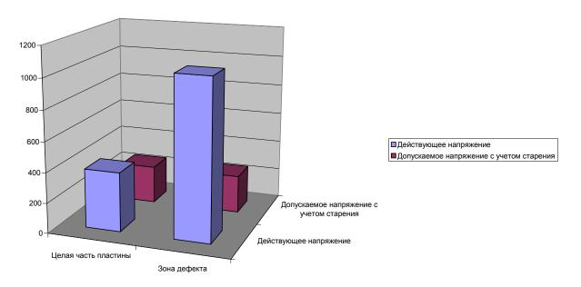
Comparison of current and voltage in the entire exfoliated composite plate with a tensile strength, calculated taking into account the aging Rules of Russian River Register.
